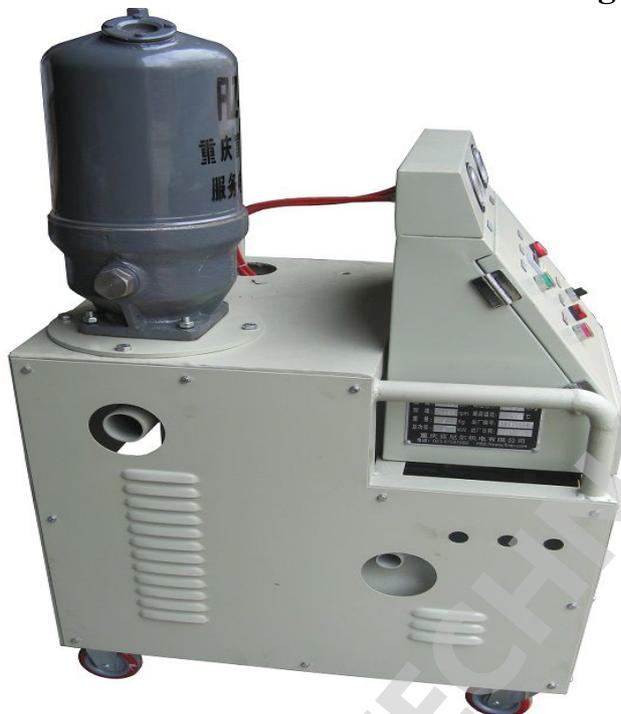
**Overview:** Centrifugal Separator is widely used in the field of wire and cable machine, especially drawing machine, to solve the aluminum wire drawing oil pollution.
