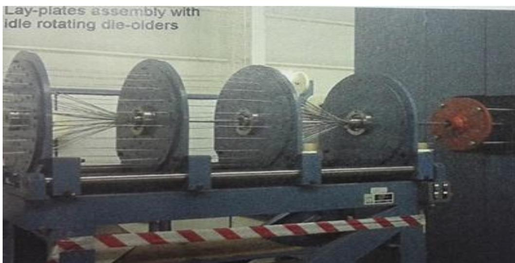
With normal aluminum wires, the high compaction degree is possible, without annealing, simply applying on-line paraffin wax.
