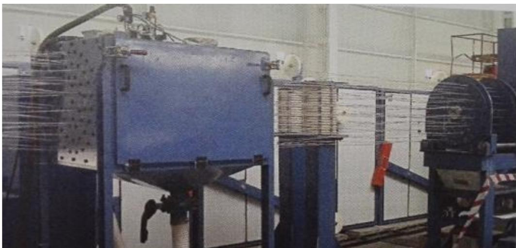
When requested, the insertion of water-swellable yarns among the layers of wires is possible. The insertion of water-swellable yarns is a special lay-plate assembly, which can be supplied by the company for the application of one or more yarns.
