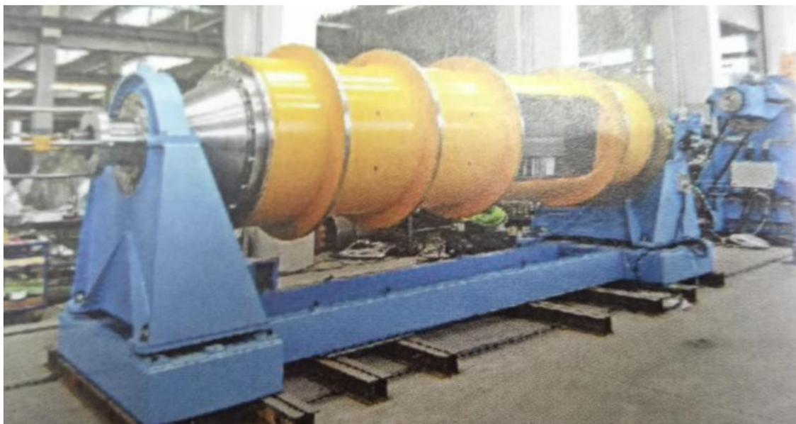
Machine that is equipped with external rotating capstan CE-1200. Same as CE-900 and :
