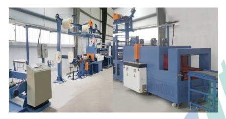
During the production of wires and cables, the packaging method in the later stage generally using a coiling, binding and film packaging. In the past, it was mainly used by a simple rewinding machine, and then wrapped films by manual. But this packaging method is mainly manual, not only has low production efficiency, high labor cost, but also it has unstable quality.
