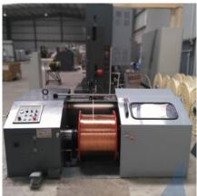
According to the requirement of the international market, we developed different types of gear type high speed medium wire drawing machine, which is similar structure to the Niehoff brand high speed drawing machine, it is suitable for drawing medium-sized copper conductors.
