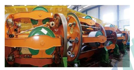
Planetary strander is an important equipment for wire and cable stranding. It is mainly used for copper stranded wire, aluminum stranded wire, steel stranded wire, steel core aluminum stranded wire, and cabling of insulated wire core and OPGW stranding, etc.
