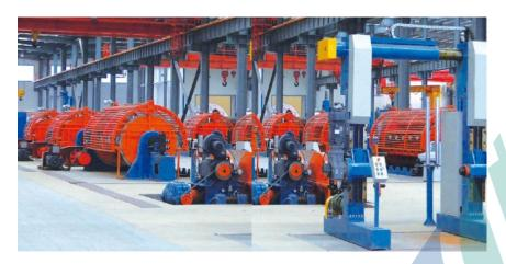
The rigid frame strander is an important device for twisting wire and cable conductors. It is mainly used for large-length, large-section aluminum, aluminum alloy stranded wire, bare copper stranded wire and steel core aluminum stranded wire, round and sector-shaped conductors, and cross-linked tightly pressed cores without back twisting.
