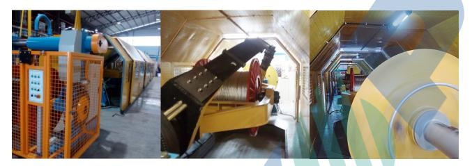
Bow twister is the important equipment for wire and cable cabling, it is mainly used for control cables, low voltage cables, rubber sheathed cables, mining cables, overhead insulated cables and other products.
