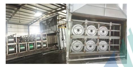
In order to improve the mechanical properties of aluminum alloy wires after drawing, quenching heat treatment is generally required. But the strength and hardness of aluminum alloy wires do not immediately increase after quenching, in order to improve the strength and hardness of aluminum alloy wire, aging treatment after quenching is required.
